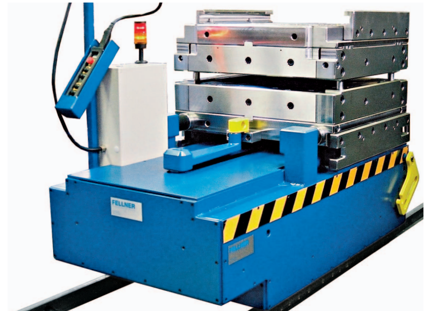
Cassette change carriage with ready-to-change rectangular forging die cassette (view from rear right)
